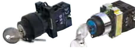
ANAHTARLI BUTON 3A / 240 V AC, IP 44
